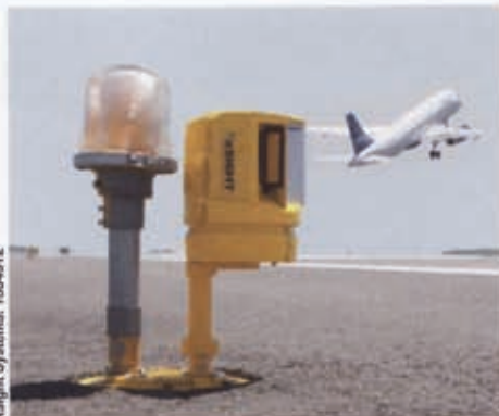
FODetect from Xsight Systems of Israel employs high-resolution cameras and millimetre-wave radars, mounted on runway edge lights. It has been tested at Boston Logan International Airport.
