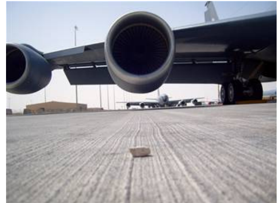
A rock sits on the flightline near an aircraft on a base at an undisclosed location in Southwest Asia. Rocks and other foreign object debris cause millions of dollars in aircraft damage each year. To deal with the problem the 379th Air Expeditionary Wing has an active FOD prevention program. (Courtesy photo)
