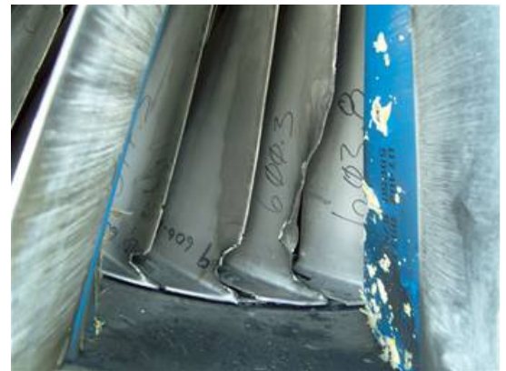
View of the front of a B-1 engine that ingested pieces of a main landing gear tire on takeoff at an undisclosed location in Southwest Asia. Repairs will cost between $260,000 and $1 million. Incidents like these highlight the need for foreign object debris prevention efforts. (Courtesy photo)
