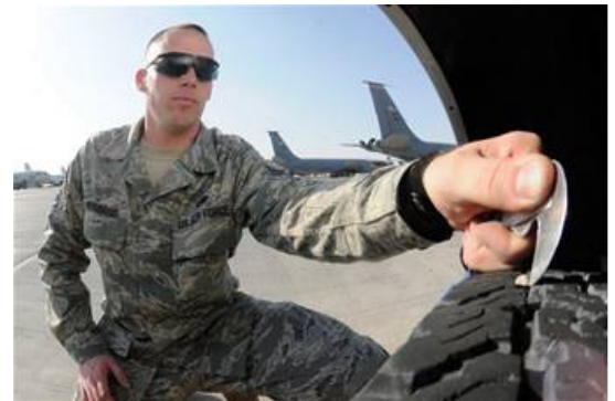
Tech. Sgt. Mark Weisbrod, foreign object damage prevention program monitor assigned to the 379th Expeditionary Maintenance Group, removes a rock from his tire using a FOD picker as part of his rollover foreign object debris check before driving onto the flight line Nov. 10, 2008, at an undisclosed location in Southwest Asia. FOD accounts for millions of dollars in damages to aircraft every year. Sergeant Weisbrod, a native of Verona, N.Y., is deployed from Dover Air Force Base, Del. (U.S. Air Force photo by Staff Sgt. Darnell T. Cannady)
